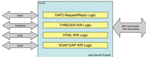
The OLFS support for DAP2 is dependent on the functions which are provided by the Back End Server (BES). When the OLFS receives a DAP2 data or metadata request, it recasts that request in terms of commands that can be sent to the BES. The BES's response is then packaged in a MIME document for transmission back to the client program.
